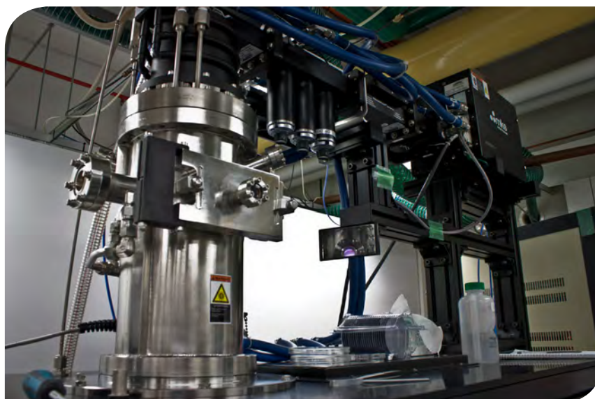
Chemical vapour deposition system (Seki AX5250) installed and running at Macquarie University
